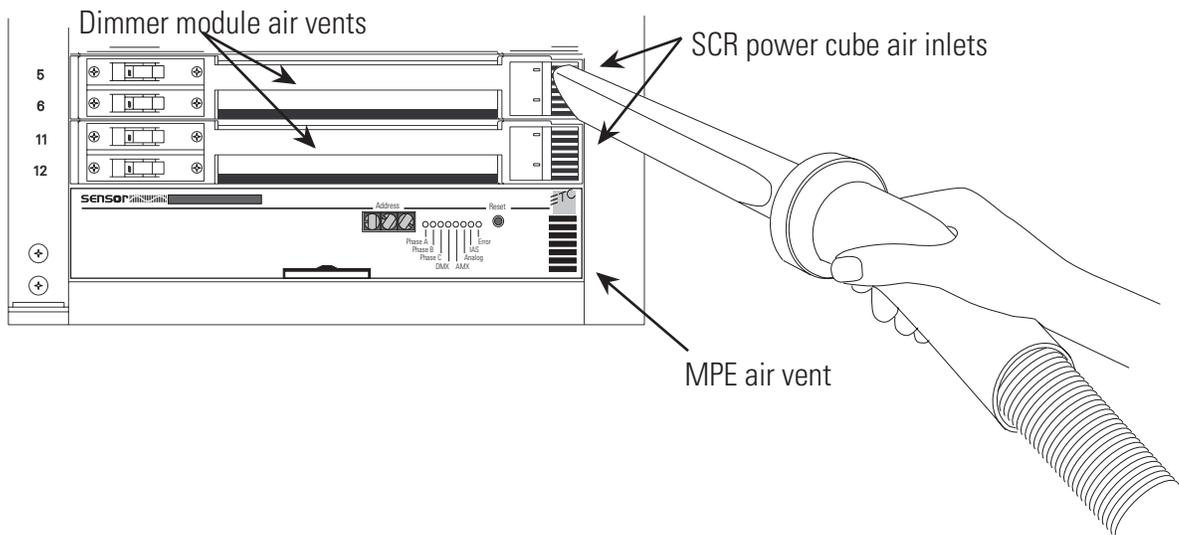
Figure 4: Vacuuming MPE rack modules
