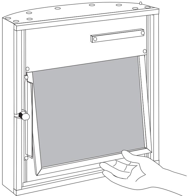
Figure 3: Removing the air filter
