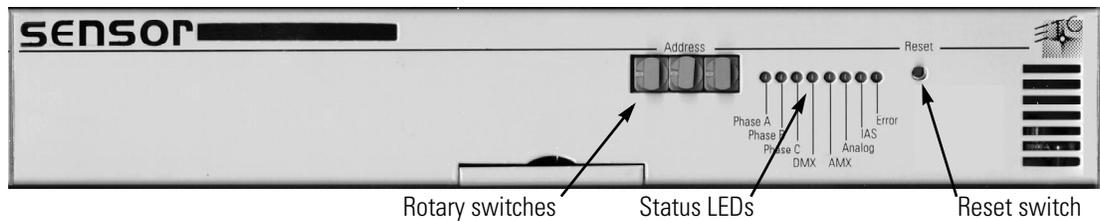
Figure 2: MPE face panel components
