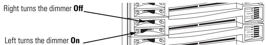
Figure 5: Dimmer module circuit breakers
