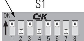
Figure 8: Configuration DIP switch settings
