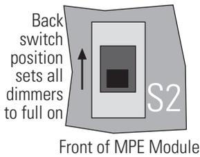
Figure 9: Test switch
