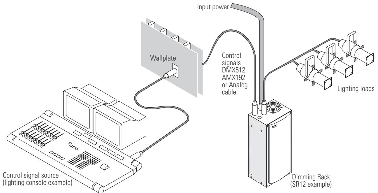
Figure 1: A typical MPE lighting system
