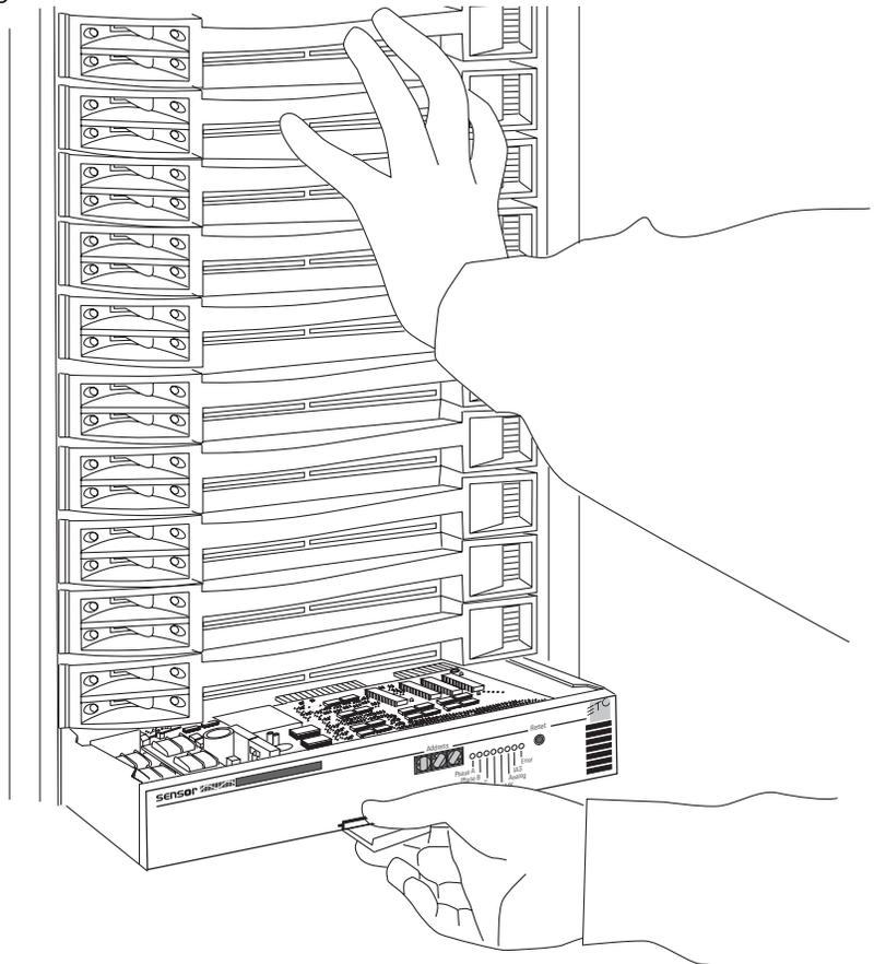
Figure 6: Removing an MPE module
