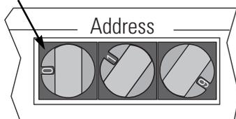
Figure 10: Setting switches
